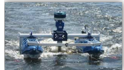
New Energy Corporation river current power generation system
